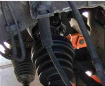
Mark the orientation of the axle to the tulip. Pull the boot back to expose the bearings. At this time verify that the splines are loose on the wheel end. if they were not, things will get ugly real fast.
